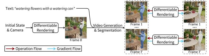
Figure 2. **Overview of ZeroHSI.** Our approach begins with HSI video generation conditioned on the rendered initial state and text prompt. Through differentiable neural rendering, we optimize per-frame camera pose, human pose parameters, and object 6D pose by minimizing the discrepancy between the rendered and generated reference videos.
